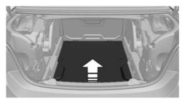
The tow fitting is located in a compartment under the cargo floor panel.
