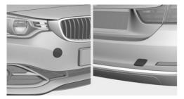
Press on the mark on the edge of the cover to push it out.
