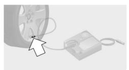
3. Attach the connection hose directly to the compressor.
