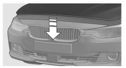
Let the hood drop from a height of approx. 16 in/40 cm and push down on it to lock it fully. The hood must audibly engage on both sides.
