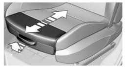
Pull the lever at the front of the seat and adjust the thigh support.
