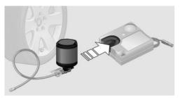
5. Screw the connection hose onto the tire valve of the defective wheel.
