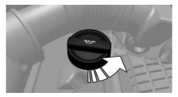
Only add engine oil when the message is displayed in the instrument cluster. The quantity to be added is indicated in the message displayed in the instrument cluster.
