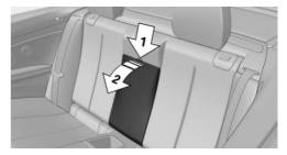
Push down the tab, arrow 1, and remove the center section, arrow 2.
