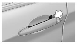
Touch the surface on the door handle of the driver's or front passenger door, arrow, with your finger and hold it there without grasping the door handle.
