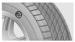
RSC label on the tire sidewall.
