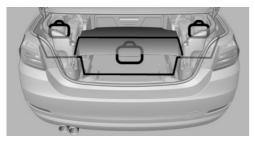
Luggage can be stowed under the trunk partition and to the left and right of the lifting mechanism; note the respective label.
