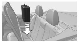
3. Fold wind deflector back and align it with the fixing point on the opposite side of the vehicle.
