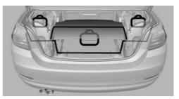
When the hardtop is closed, objects can be placed in the area below and next to the cargo area partition.
