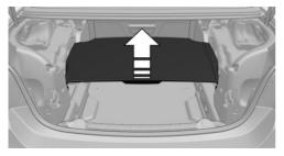
With the hardtop closed, the cargo area volume can be expanded. To do this, push the cargo area partition upward.
