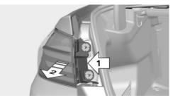
5. Release the catch at the top on the connector of the connecting line and remove the connector from the bulb holder.
