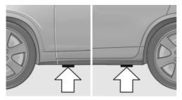
The jacking points for the vehicle jack are located at the positions shown.
