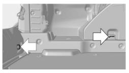
To secure the cargo there are four lashing eyes in the cargo area.
