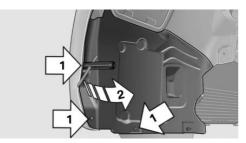
Pull off the bulb connector, arrow 1. Turn the bulb, arrow 2.
