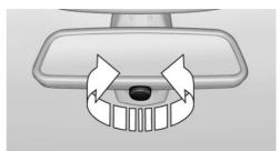
Turn the knob to reduce the blinding effect by the interior mirror.
