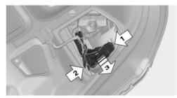
2. Loosen the top holder, arrow 2. To do so, press in the middle latch and then press out both outside latches.
