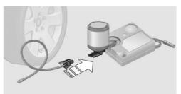
4. Slide the sealing container upright into the holder on the compressor housing, ensuring that it engages audibly.
