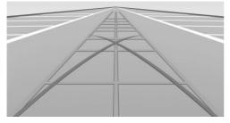
2. Turn the steering wheel to the point where the pathway line covers the corresponding turning radius line.
