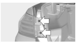
4. Grasp the inner edge of the tail lamp, arrow 1, and carefully pull it backward and out, arrow 2. Use your free hand to hold it in place in order to prevent the tail lamp from coming loose suddenly. Make sure that the foam rubber sealing ring is on the centering pin.
