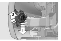
3. Insert the new bulb, connect the connector and screw on the wheel house panel.
