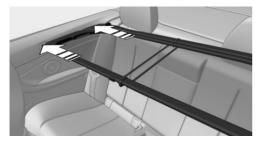
5. Press the wind deflector inwardly and up, arrow 1, to the extent that the wind deflector can be positioned in front of the fixing points on the installation side.
