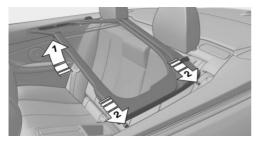
6. To ensure safe latching, press the wind deflector downward in the middle, arrows 1.
