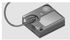
4. Insert the connector into a power socket inside the vehicle.
