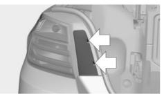
3. Loosen the two nuts with the screwdriver handle, arrows.
