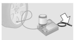
7. With the ignition turned on or the engine running, reel on the compressor.
