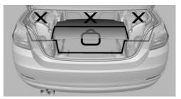
When the hardtop is open, objects can be placed below the cargo area partition. Do not use the areas marked X in the illustration as storage areas.
