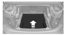
The first aid kit is located in a compartment under the cargo floor panel.
