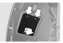
2. If necessary, pull the inside trim of the wheel house slightly inward. Turn the bulb socket counterclockwise and remove.
