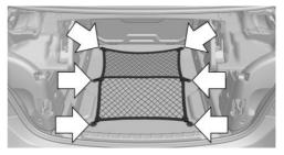
Hook the floor net into the fittings in the trunk floor.
