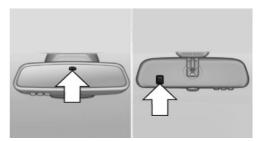
Photocells are used for control:
