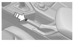
Raise lever slightly, press the button and guide the lever down.
