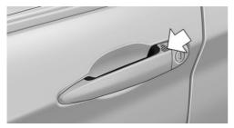
Touch the surface on the door handle of the driver's or front passenger door, arrow, with your finger for approx. 1 second without grasping the door handle.
