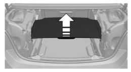
Fold down trunk partition in the back so that the hardtop can be opened.
