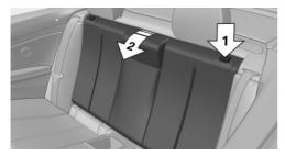
Unlock the rear seat backrest, arrow 1, and fold forward, arrow 2.
