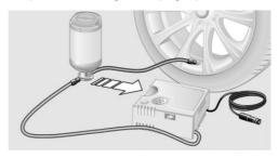
Screw the filling hose of the sealant container onto the tire valve of the nonworking wheel.
