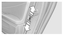
Push the locking lever on the rear doors down.
