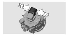
5. Turn the bulb bracket and remove it.
