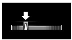
The mark in the efficiency display is backlit in blue and is located at the zero point. The tachometer approximately indicates idle speed.
