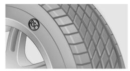
RSC label on the tire sidewall.
