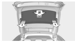
Push the cargo cover upwards, arrow 2, and remove it.
