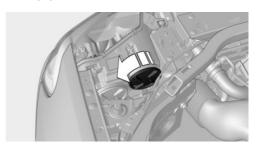
The upper bulb is the high beam/headlight flasher and the lower bulb is the daytime running lights.
