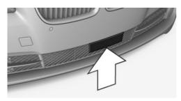
Always keep radar sensor clean and unobstructed.
