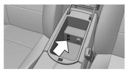
An external audio device, e.g., an MP3 player, can be connected via the AUX-IN port in the center armrest.
