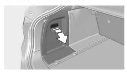
The onboard vehicle tool kit is located under the first-aid kit behind the left folding cover in the trunk.
