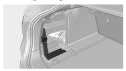
The warning triangle is located behind the lefthand cover in the trunk.
