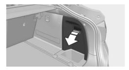
Open the cover on the right side trim, arrow, and remove the sound insulation.
