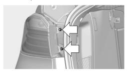
Remove the tail lamp from the body and detach the connector from the bulb holder.
