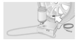
With the compressor switched off, insert the plug into the power socket inside the vehicle.
