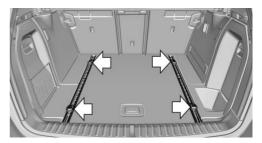
To secure the cargo there are four movable lashing eyes in the cargo area.
