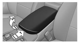
Press button, arrow 1, and fold the center arm rest up, arrow 2.
