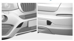
Press on the mark on the edge of the cover to push it out.
