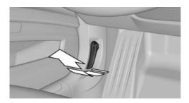
Press the release handle and open the hood.
