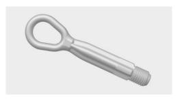
The screw-in tow fitting should always be carried in the vehicle.
