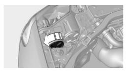
3. The upper bulb is the low beam and the lower bulb is the parking lamp.
