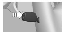
Press and hold PC button on blinker lever.
