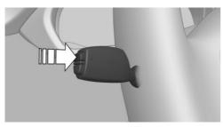
Press and hold PC button on blinker lever. Information is displayed in the info display of the instrument cluster.
