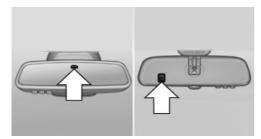
Photocells are used for control:
