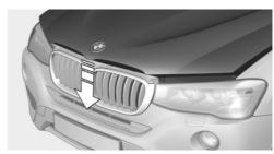
Let the hood drop from a height of approx. 16 in/40 cm and push down on it to lock it fully. Make sure you hear the hood engage.
