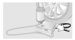
7. With the ignition turned on or the engine running, switch on the compressor.
