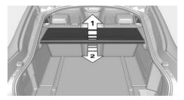
Push the cargo cover upwards, arrow 1, until it disengages from the catches and then pull it towards the front, arrow 2.
