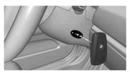
Steptronic transmission: if a corresponding Check Control message appears, hold the remote control, as shown, against the marked area on the steering column and press the Start/Stop button within 10 seconds while pressing the brake.
