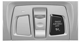
The indicator lamp for the front-seat passenger airbags indicates the operating state of the front-seat passenger airbags.
