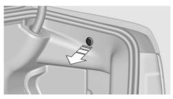
Pull the green knob with the fuel pump symbol. This releases the fuel filler flap.
