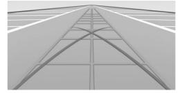
2. Turn the steering wheel to the point where the pathway line covers the corresponding turning radius line.
