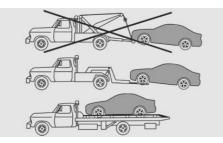
Have your vehicle transported with a tow truck with a so-called lift bar or on a flat bed.
