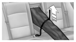
Securing the ski bag Secure the ski bag by tightening the retaining strap; otherwise, the contents could present a source of danger to the passengers, for example during braking or evasive maneuvers.
