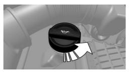
Only add engine oil when the message is displayed in the instrument cluster or when the engine oil level has almost dropped to the lower mark of the dipstick.
