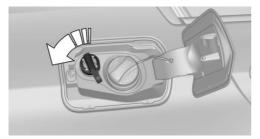
The tank for the reducing agent is located next to the fuel tank.
