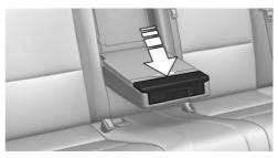
The cupholder can be adjusted for three different container sizes.
