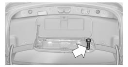
The tow fitting is located in the container on the inside of the trunk lid.
