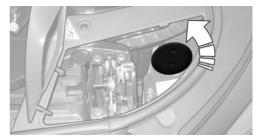
3. Unscrew the bulb holder counterclockwise.
