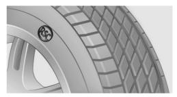
RSC label on the tire sidewall.
