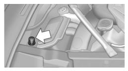
The body ground or a special nut acts as the battery negative terminal.
