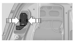
Squeeze the clips together and remove the bulb holder.
